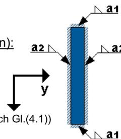
**Naht 2:** max.Sigma<sub>⊥</sub> = 8,25 kN/cm<sup>2</sup>
